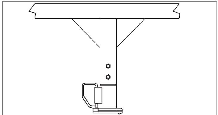
We have utilized a ball receiver that is suitable for the size and weight of the trailer. The load rating of the receiver and the necessary ball size are listed on the gooseneck.
